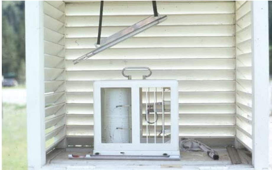
Figure 9. Hygrothermograph mounted in separate screen with double-louvered sides and double roof. Photo courtesy of British Columbia Ministry of Forests and Range, Protection Branch.
