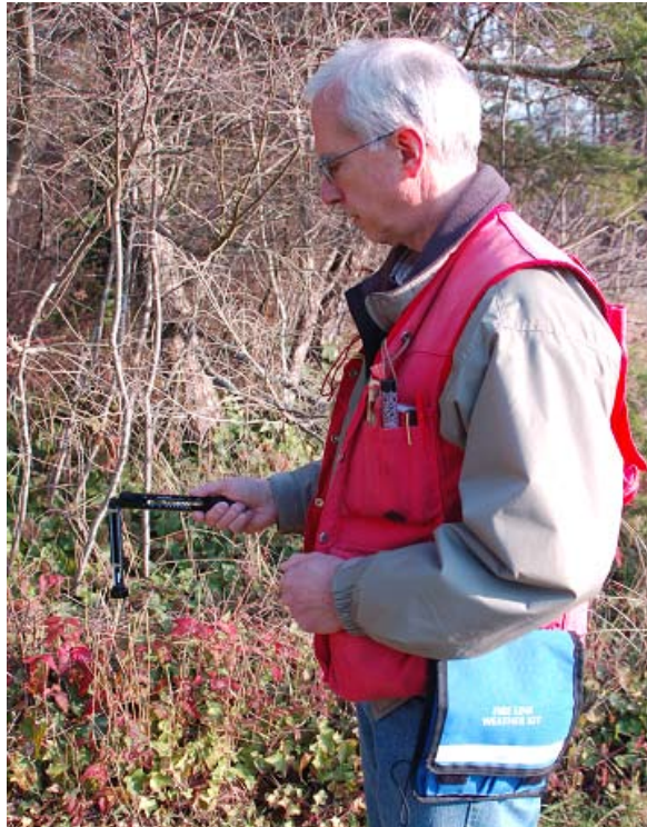
Figure 17. Sling psychrometer from belt-mounted weather kit used for local measurements of wet-bulb and dry-bulb temperatures and calculation of relative humidity (photo courtesy of Ember Research Services Ltd.).
