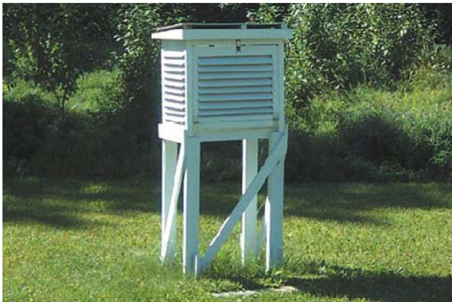
Figure 7. Stevenson screen, on an open framework stand that is staked to the ground. The floor of the unit is 115 cm above ground. The white-painted double-louvered wooden door faces north on this unit, which is located in the northern hemisphere. Photo courtesy of British Columbia Ministry of Forests and Range, Protection Branch.
