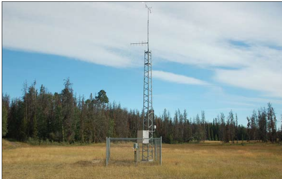
Figure 6. Fire weather station in large clearing on open level ground. Photo courtesy of Ember Research Services Ltd.
